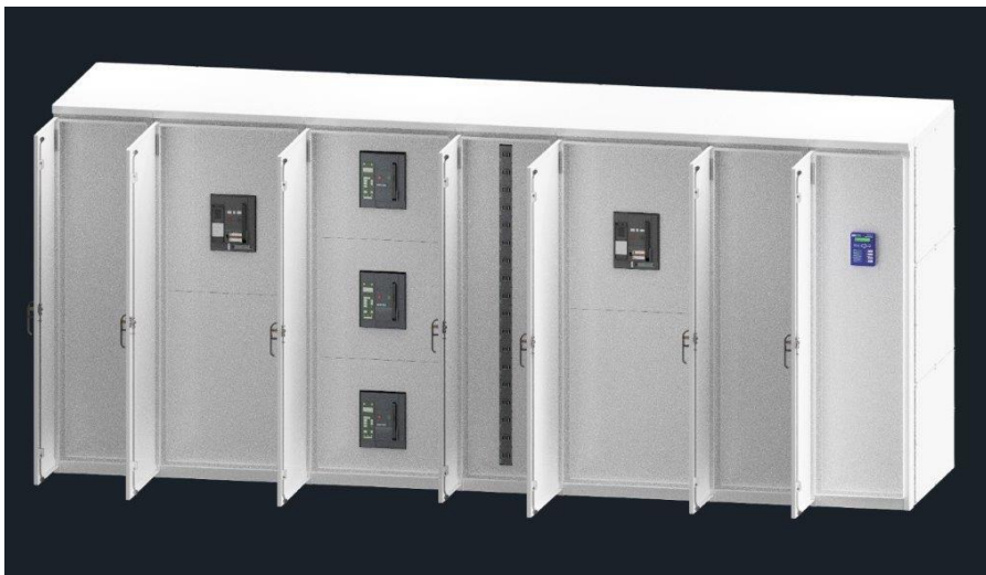
Pictured left: UL 891 / NEMA 3R 480 / 277VAC, 1200-5000A SWBD, with: cable input section, 5000A main, ACB feeder section, MCCB feeder section, 2 nd main section, 2 nd main input section & SEL control section.
