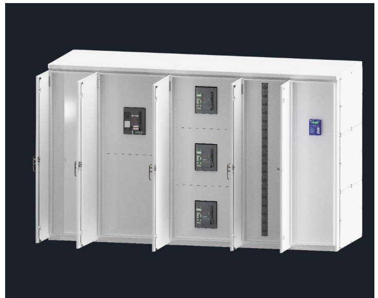
Pictured above: UL 891 / NEMA 3R 480 / 277VAC, 1200-5000A SWBD, with: cable input section, 5000A main, ACB feeder section, MCCB feeder section & SEL control section.
