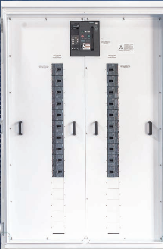
1600A to 4000A NEMA 3R SWBD with main and up to 30 feeders, deadfront view.
