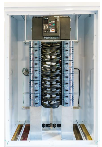
Pictured above: UL / NEMA 3R 480 / 600VAC, 4000A bus, 4000A main with qty (20) 150AF MCCB feeders
