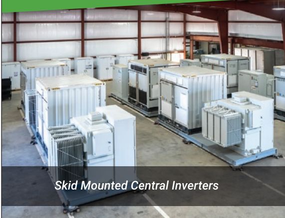
Fully Factory Intergrated Skid Mounted PV Unit Substations (XFMR, SWBD, Aux Power and SCADA)
