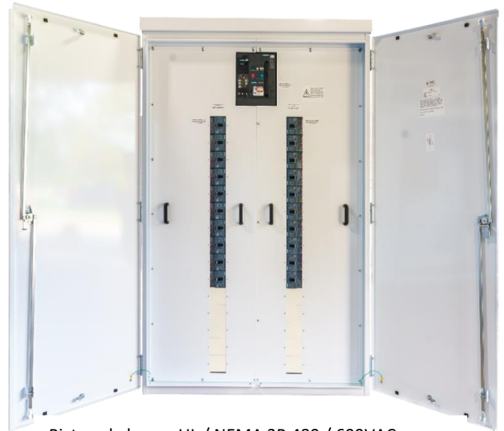
Pictured above: UL / NEMA 3R 480 / 600VAC, 4000A bus, 4000A main with qty (20) 150AF MCCB feeders
